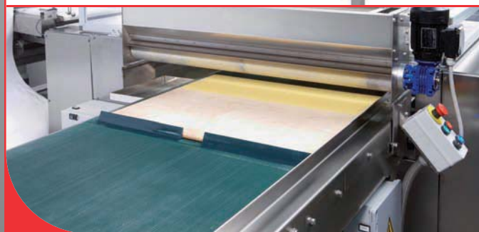
Reciprocating Belt Panner with a tray feeding cross conveyor, complete with a corn meal duster to dust the peelboards before panning.
