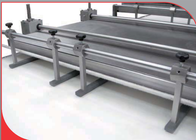
Lateral bar to close the ends of the baguette or finger rolls and give them the same size.
